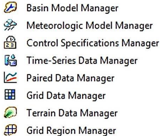
Figure 5. Components of the HEC - HMS hydrological modeler. Source: Own elaboration.
